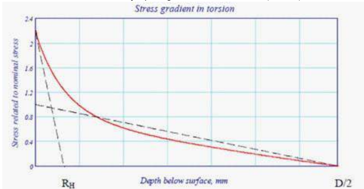
Figure 18 : Torsional SCF in the crankpin fillet as a function of depth. The corresponding SCF for the journal fillet can be found by replacing R_H with R_G and D with D_G (1/7/2018)
