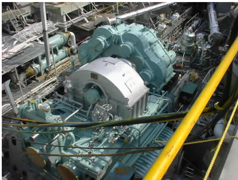
Figure 5.3: Traditional Steam Plant Layout
